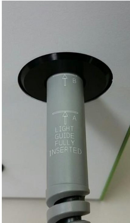
Figure 4 Correct position for fully inserted X-Cite LLG with A and B insertion lines
