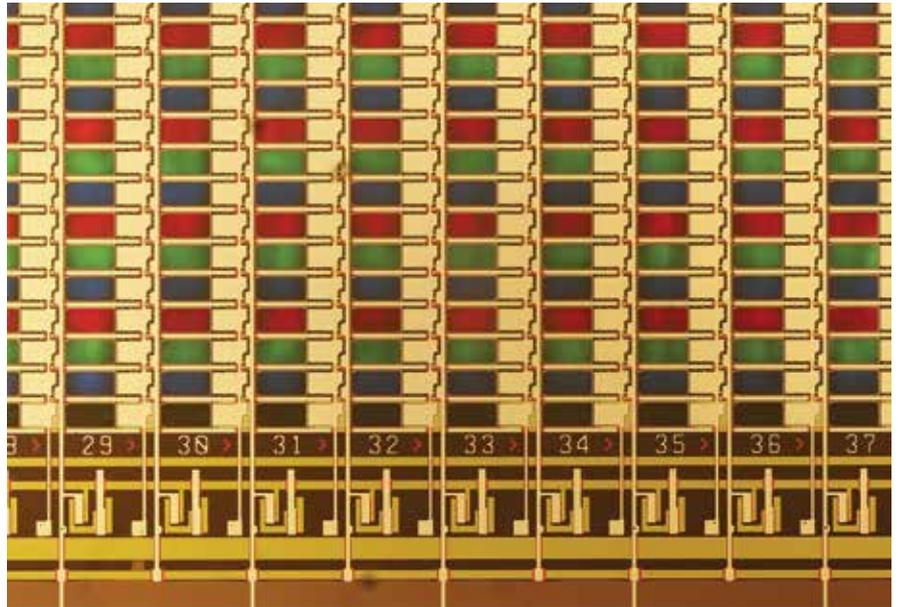
Flat panel inspection requires optics with excellent color correction for individual inspection of red, green, and blue pixels, without the need to refocus, regardless of which pixel color is active.
