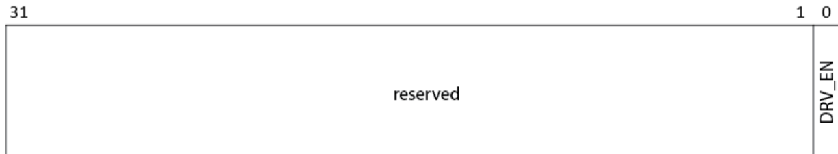
Figure 23 Motor Driver Control
