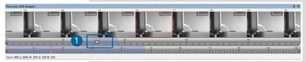
Clicking (left mouse button) within the upper scale bar 1, you can adjust the number of images which are shown by moving the mouse left or right. Minimum is 20 and maximum is half of the recorded images in this scale.
