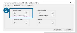
Check if **GPU Processing** is activated by having a look into the **Proc config** settings 2 in the **Convert Control** window 1 (see pco.camware manual).
