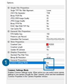
If you work with the pco.dicam C4, the *Common Properties* help to simplify the recording setup by determining which settings are common to all four cameras and which are set individually for each individual camera.
