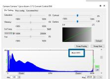
Try to adjust the amount of illumination so that about 25% of saturation level (16.000 counts) are achieved as a mean value. Compare the mean values of all four channels.
