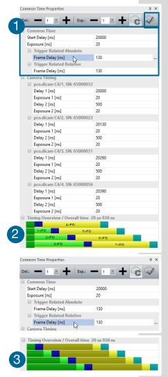
How to configure the timing for all channels in double image mode with *Common Time Properties* is explained in this chapter. This mode is recommended for the pco.dicam C4 for the most common application scenario where 8 identical exposure times shall be equidistantly positioned on the time line corresponding to a constant fps.
