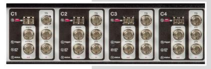
For single triggering, a BNC socket (plus arm socket for double image operation) is available on each channel for electrical triggering.
