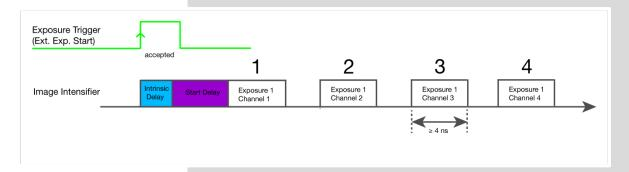
This diagram shows a single four image burst using *Master Trigger*.
