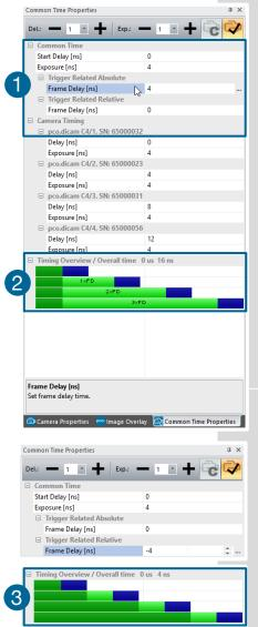
How to configure the timing for all channels in single image mode with *Common Time Properties* is explained in this chapter. This mode is recommended for the pco.dicam C4 for the most common application scenario where 4 identical exposure times shall be equidistantly positioned on the time line corresponding to a constant fps.
