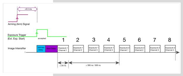
for a single eight image burst using Master Trigger
