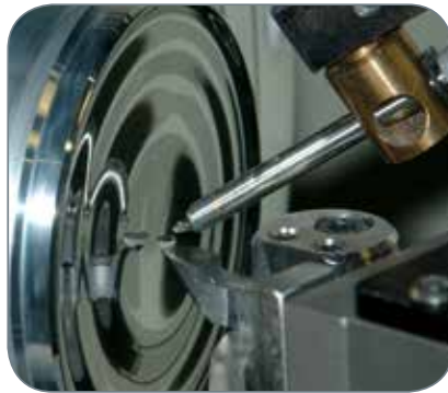
Rotation-symmetric multiple aspherical surface, aluminium.
