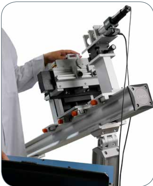
Application example: A measuring station for determining geometric parameters of cylindrical lenses built by OEG GmbH out of X95 components.
