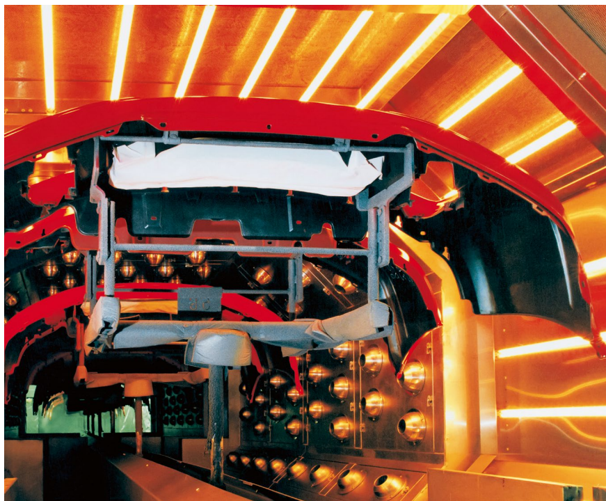
An infrared system in front of a hot-air oven dries coatings on plastic bumpers much faster.
