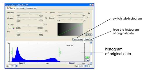
The user can influence how the 12 bit intensity values (x-axis) of the original image are converted into 8 bit values (y-axis) in different ways.
