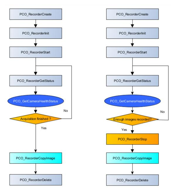
The left workflow is similar to the first example in section <u>3.2</u>. It uses **PCO\_RecorderGetStatus** to wait for the acquisition to finish. This is a default approach for **PCO\_RECORDER\_MODE\_FILE** and **PCO\_RECORDER\_MODE\_MEMORY** with type sequence (see chapter **2.7.1**).
