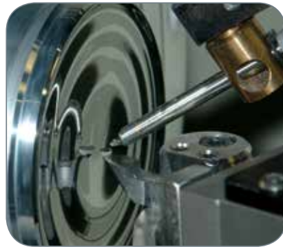
Rotation-symmetric multiple aspherical surface, aluminium.
