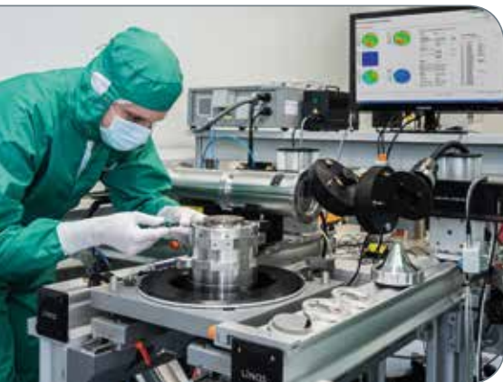
X95 table construction for an assembly of complex optical systems in a clean room at Qioptiq in Göttingen.
