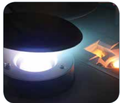
Coating unit for plasma assisted vapour deposition
