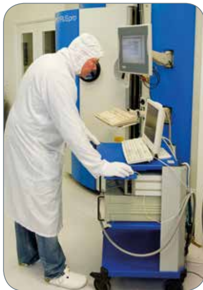
Parameter setting and start of the coating process
