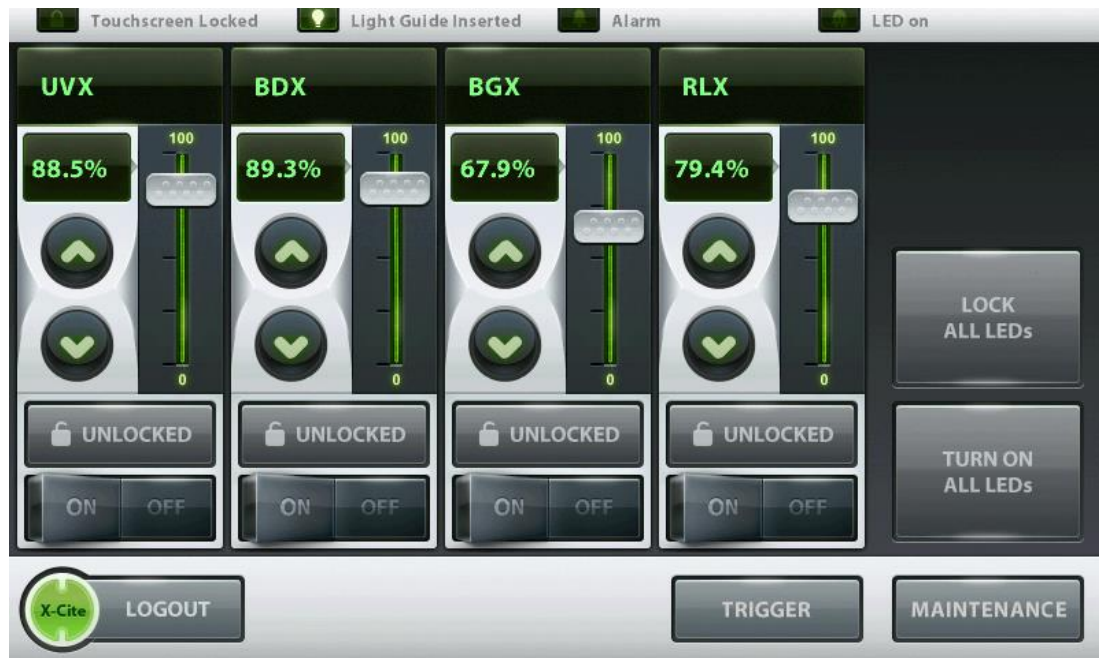
Figure 21 Main LED Screen (Touch Screen Controller)
