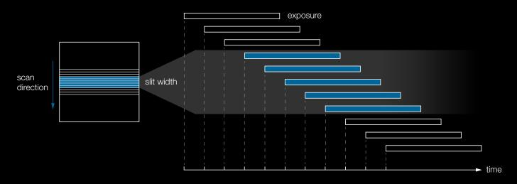
Exemplary illustration of the readout in lightsheet scanning mode with five exposure lines. This corresponds to a slit width of five times the pixel height.
