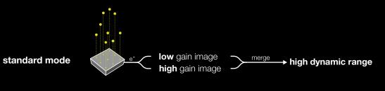
The low light mode benefits from two times correlated multi sampling of high gain images. This reduces the temporal noise by a factor of the square root of 2, which is ideal for applications demanding low noise and high sensitivity.
