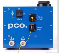
First connect the **Power out** of the cooling unit with the **Power in** of the pco.flim camera by using the PCO WAT camera cable. Or use separate power supplies for camera and aquamatic.
