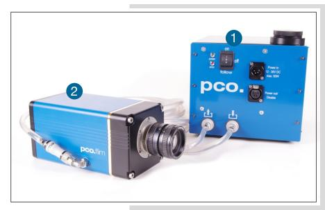
This is the re-cooling system for pco cameras with water-cooling.
