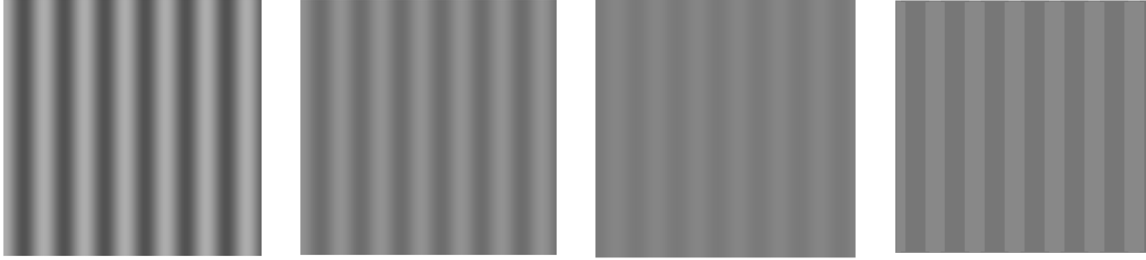
Figure 3. The left figure shows the in-focus image of the sinusoidal mask. The other images correspond to normalized defocus settings of u = 5, 10, 15 .
