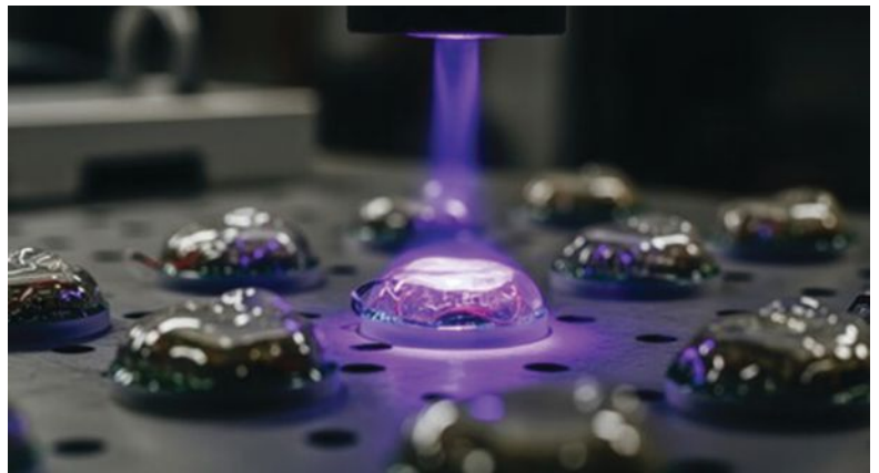
Figure 1. Spot curing allows precise control of UV exposure.
