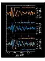
Plots of Excelitas Photodiode readings show the gravitational wave disruption on the beams at both Livingston and Hanford LIGO facilities only thousandths of a second apart, and then superimposed against Einstein's original predictions (*image courtesy of Caltech/MIT/LIGO Laboratory*). Click here to download high-resolution image.
