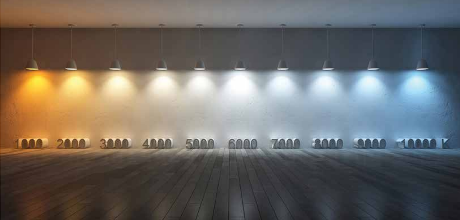
Figure 2. Depiction of a CCT (correlated color temperature). Warm-colored red-orange sources have lower temperatures (kelvin) than cool-colored blue-white sources. Modern LED systems for endoscopy allow users to adjust the level of each visible color to their comfortable CCT level, which reduces eyestrain.
