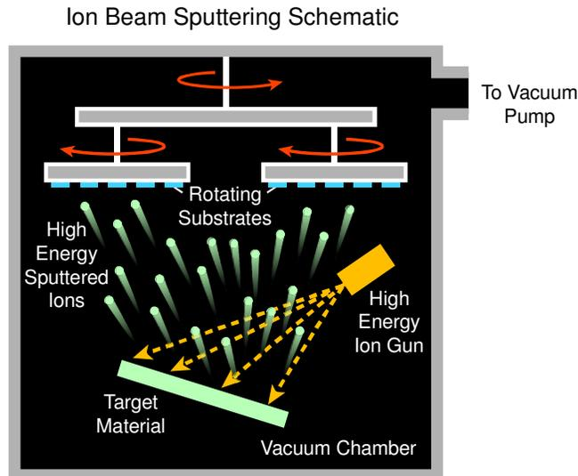
*In IBS, a high energy ion beam is directed at a target causing atoms or molecules to sputter off with high energy, resulting in densely packed films.*
