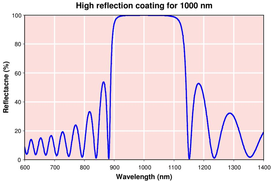
*Reflectance of a typical narrowband high reflector coating, in this case centered at 1000 nm.*
