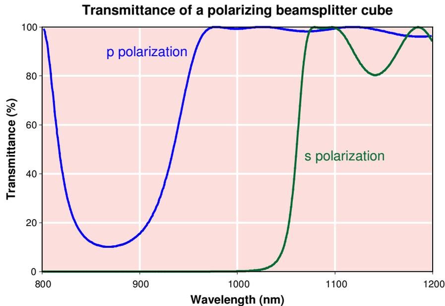
*Polarizing coatings maximize the difference in reflectance between  $s$  and  $p$  polarizations to achieve high extinction ratios.*
