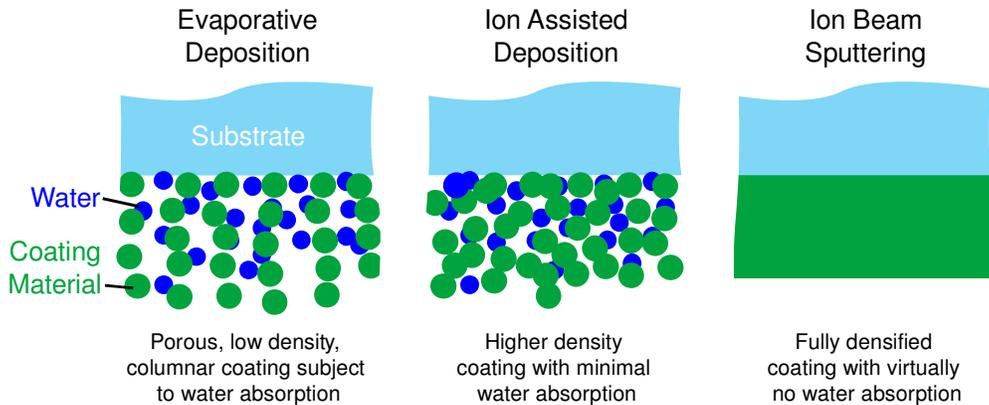
*Evaporative deposition produces porous coatings which can absorb moisture, while IAD reduces this problem and IBS completely eliminates it.*
