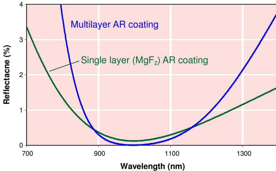
*Adding layers to an antireflection coating lowers the reflectance but reduces the coating bandwidth.*
