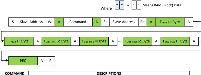
Block Read RAM, from Address 18 (T<sub>AMB</sub>) to Address 26 (T<sub>OBJ PIX8</sub>)
