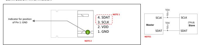
NOTE 1: The SCLK and SDAT pins are open collector. Apply appropriate pull up resistors (e.g. 4.7 kOhm) on the SMBus master device.
