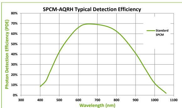
Figure 3. Typical Photon Detection Efficiency (PDE) vs. Wavelength
