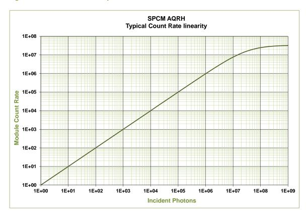
Figure 8. Optical Power vs. Number of Photons
