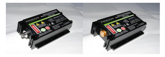
SPCM with free space window (right) and with FC adaptor (left), for tube cage mount bracket and C-mount bracket see page 11
