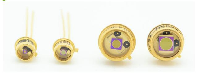
Excelitas' Large Area PIN Diodes are highly sensitive, low capacitance InGaAs diodes that provide high responsivity from 800 nm to 1700 nm. An ultra-low capacitance version for high bandwidth applications is available upon request.
