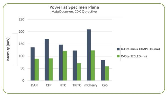
Power comparison at specimen plane using standard filter cubes. X-Cite mini+ exceeds the performance of X-Cite 120LEDmini across the visible spectrum.
