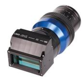
Featuring an f/2.4 aperture, the inspec.x HR 2.4/128 3.33x Lens maintains outstanding imaging quality with high-intensity light throughput. It also achieves extremely low distortion of less than 0.1% across the entire image circle. The HR 2.4/128 3.33x's spectral range of 400nm-750nm is precisely suited for use with modern, high-resolution 12k and 16k line cameras supporting 3.5 µm and 5µm sensors.
