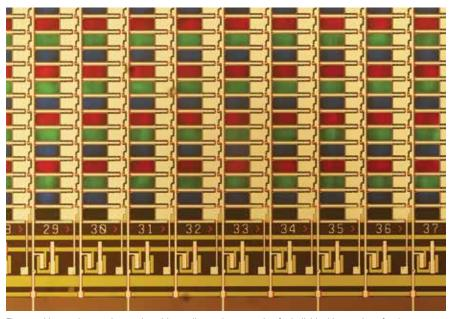
Flat panel inspection requires optics with excellent color correction for individual inspection of red, green, and blue pixels, without the need to refocus, regardless of which pixel color is active.
