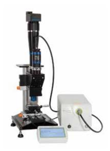
This system illustrates a highly specialized fusion between inspection optics and a microscope, enabling inspection with submicron resolution across large fields of view.
