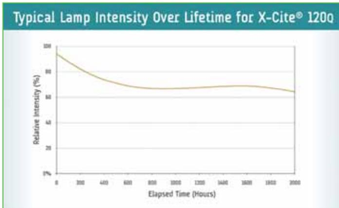
Fig. 1 – Intensity decay of an arc-lamp over 2000 hours
