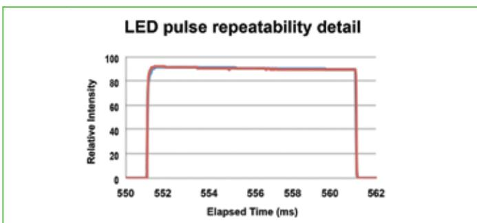
Fig. 7b - Intensity of each 10ms pulse (from fig. 7a) over 10 minutes, overlaid onto one graph.
