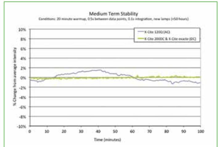
Fig. 2b – AC vs DC lamp stability over 120 minutes
