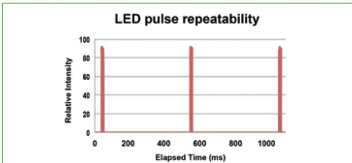
Fig. 7a - X-Cite XLED1 10ms pulse repeatability over 10 minutes.
