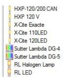
Choose your light source and double click it to insert it to your active configuration. Configure the COM port to match the port number the device was enumerated to during installation, number 4 in this case.
