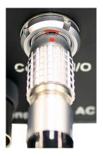
Figure 5: Removal of Control Cable.
