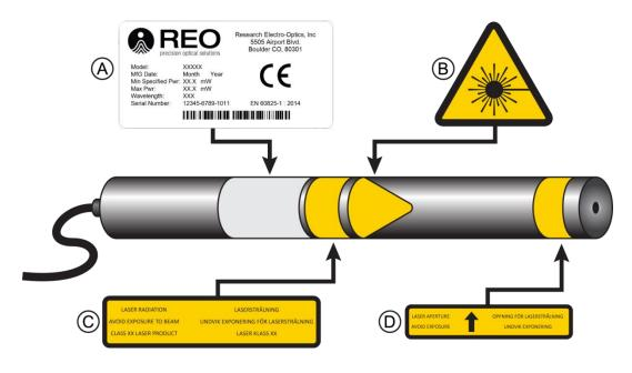
Figure 1: Laser Head Label Placement Diagram
