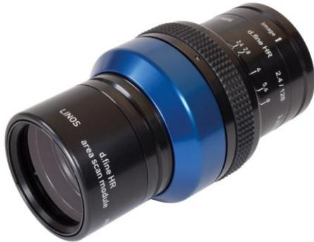
Made in Germany, the d.fine HR Lens and its Area Scan Module offer brilliant optical performance. Due to the extremely high resolution in the object of up to 300 Lp/mm and its exceedingly large image circle of 82 mm, the d.fine HR Lens with Area Scan Module accessory can be used with common area scan cameras over 150 MPixel and pixel sizes down to 3.5µm for optical inspection.
