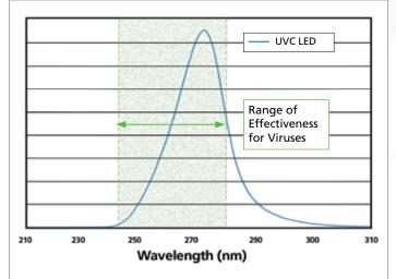
**UVC LED Spectral Output vs. Disinfection Bands**
