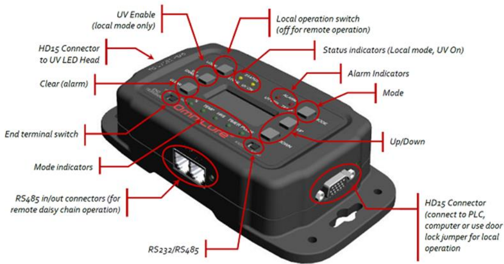
Figure 2 Console automate programmable PLC
