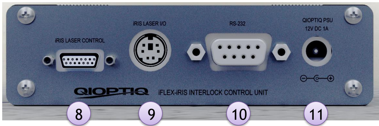
Figure 2-10: Rear panel view of the iFLEX-iRIS™ Interlock Control Unit detailing the location of the different connectors
