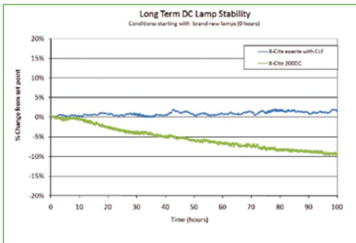
Fig. 3 – DC lamp intensity change with and without closed-loop feedback over 100 hours
