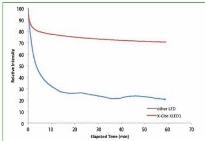
Fig 5 – Intensity drop and stabilization of X-Cite XLED1 vs. another LED unit
