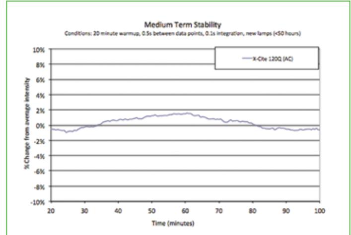
Fig. 2a – AC lamp stability over 120 minutes
