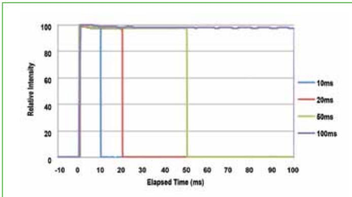
Fig. 6 – X-Cite XLED1 intensity stability over various exposure times
