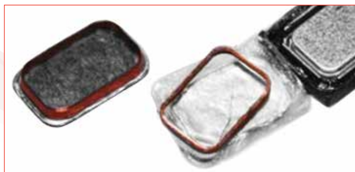
FIGURE 3: Bonding of the voice coil to the heat dissipating cover.
