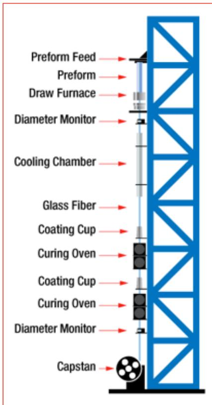
FIGURE 1: Schematic of a fiber optic drawing tower.
