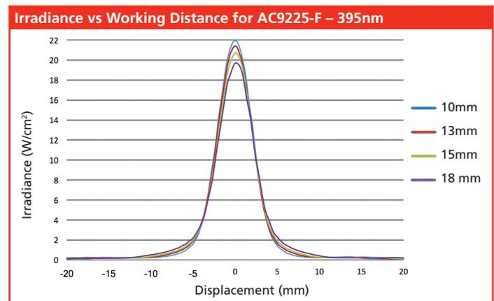
Typically, an LED curing system is very sensitive to the working distance, where the irradiance level will change significantly with small changes to the working distance. The custom optics of the OmniCure AC9225-F system maintain the irradiance almost unchanged from 10 to 18 mm, the typical working distances for the fiber coating application.
