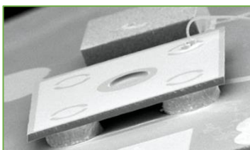
Image 4 – The SLiK Avalanche Photodiode, optimized for single photon detection
