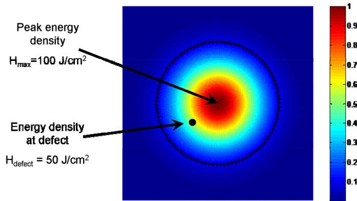
Figure 8. Knowing the precise location of the defect relative to the beam center, together with a calculated spatial profile of the beam (using measured beam parameters), allow the actual fluence at the defect to be calculated.
