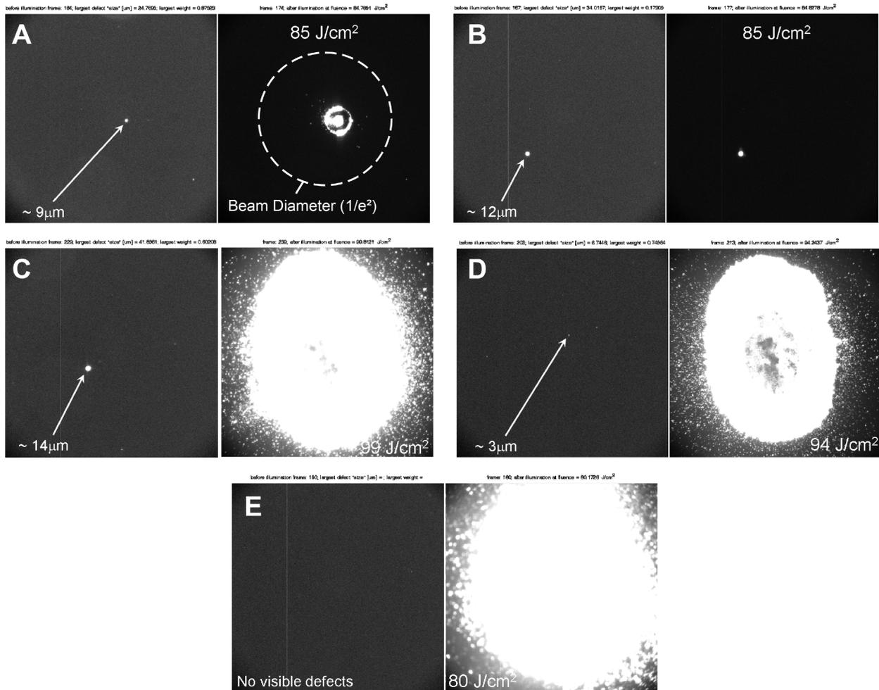
Figure 7. Photos of five regions on various components before and after laser damage testing (all at the same scale). The incident fluence at the center of each region pictured is noted, and the input beam diameter is indicated in photo pair A.
