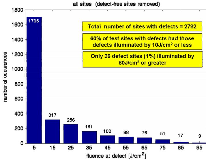
Figure 10. Histogram of the actual fluences at the defect sites.
