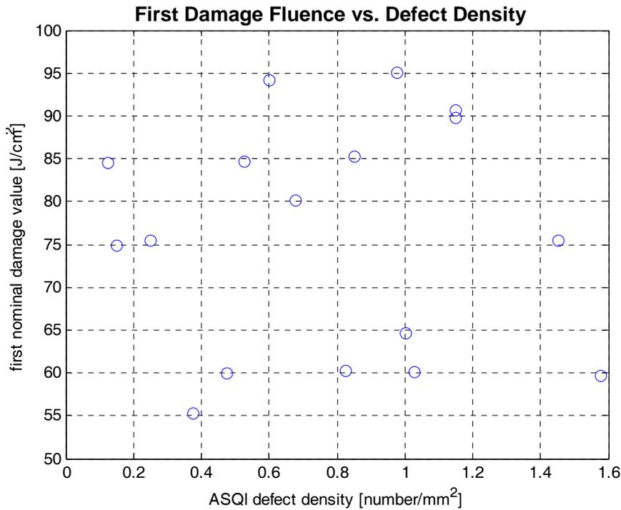
Figure 6. A plot of first damage fluence vs. defect density shows no correlation.
