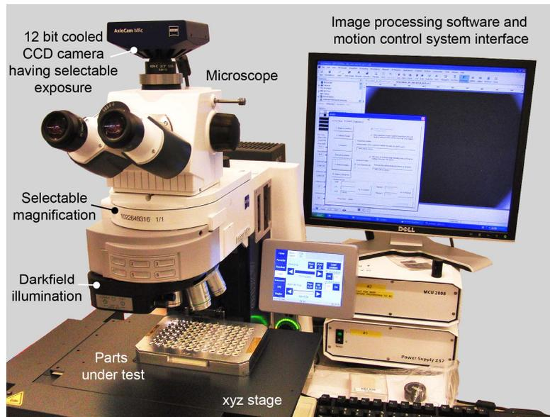
Figure 2. An automated surface quality inspection (AQSI) system which utilizes a microscope optical system and CCD camera to measure the brightness of light scattered from defects under darkfield illumination conditions.
