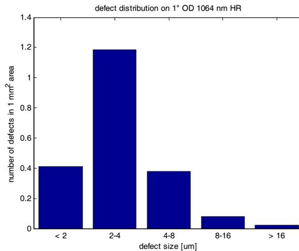
Figure 4. Histogram showing the size distribution of over 4000 defects identified by the AQSI on the 50 components under test.
