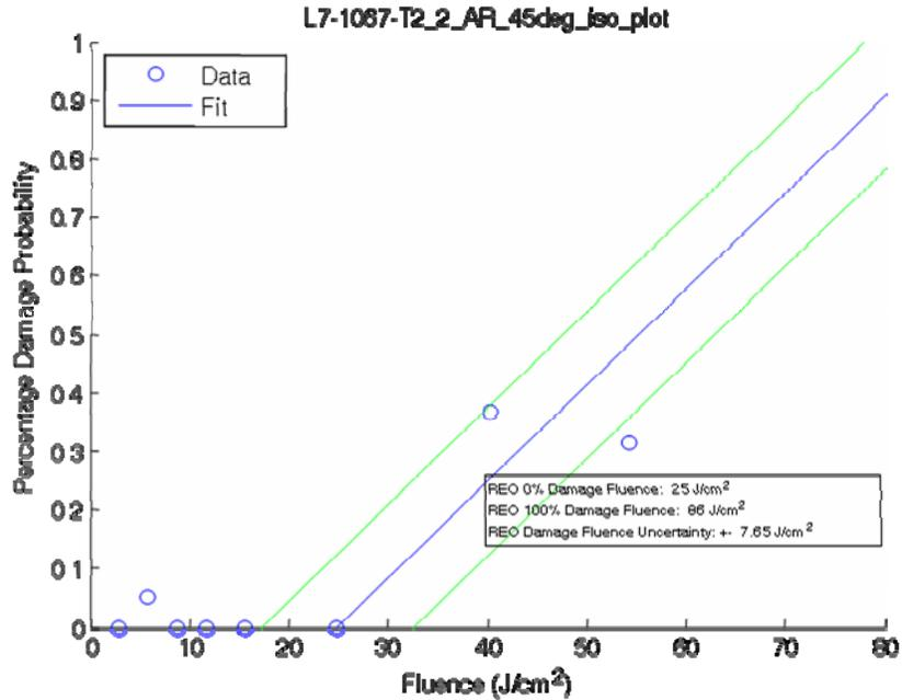
Figure 1. Laser damage threshold testing results for a single component exposed to fluences over the 2 J/cm<sup>2</sup> to 55 J/cm<sup>2</sup> range.
