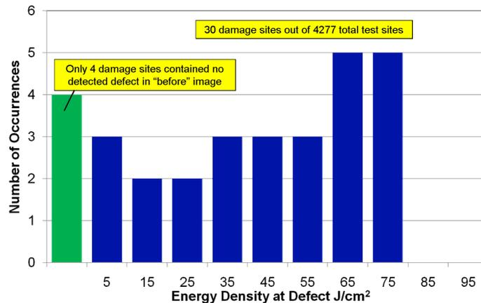
Figure 9. Histogram of the number of damage events for each fluence level at the defect.
