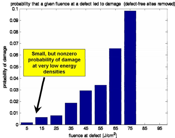
Figure 11. A normalized histogram of damage probability vs. fluence.
