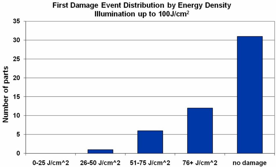
Figure 5. Histogram showing the “first damage event” results for the 50 components under test.
