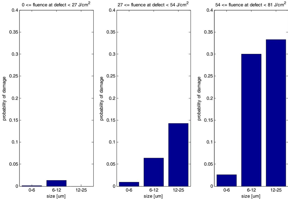
Figure 12. Damage probability vs. defect size, binned by energy density range.
