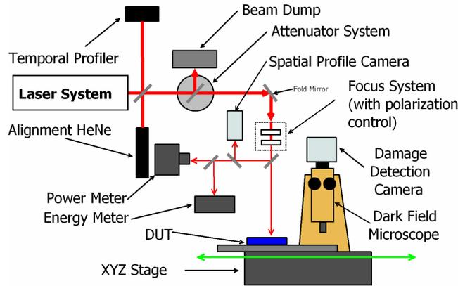
Figure 3. Schematic of the experimental setup used for laser damage threshold testing.
