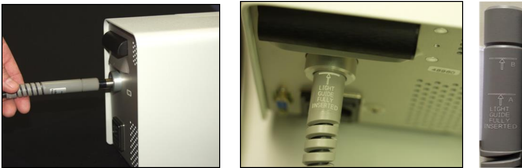
Figure 9 Light Guide Insertion
