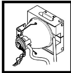
6. Locate the 4-pin Intelli-Lamp sensor connector at the rear of the lamp module and connect it to its mate located on the top of the lamp-housing wall.
