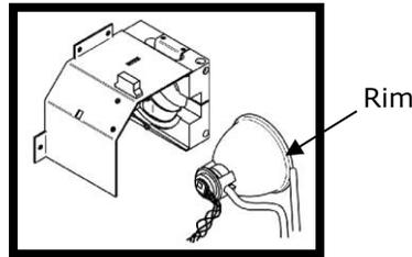
**Caution:** Do not touch the bulb's glass envelope or the inside surface of the reflector. Skin oils can cause the lamp module to fail prematurely.
