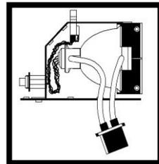
**Tip:** the Intelli-lamp connector will only attach in the correct orientation. If you are having difficulty attaching the connector, try rotating it by 180°.
