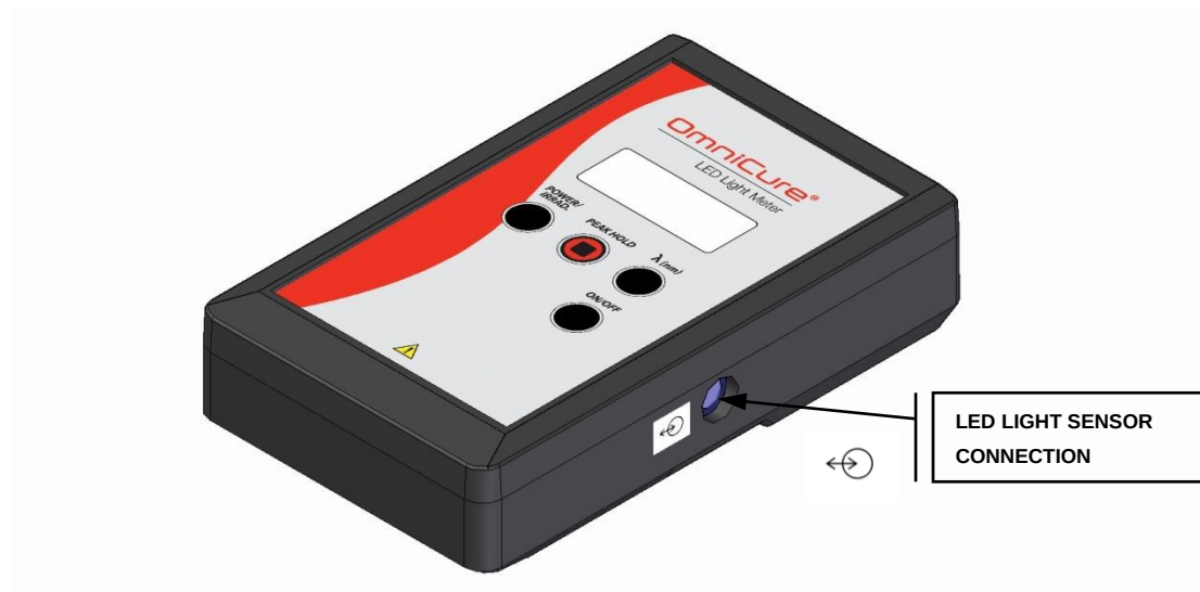
Figure 2 LED Light Sensor Connection
