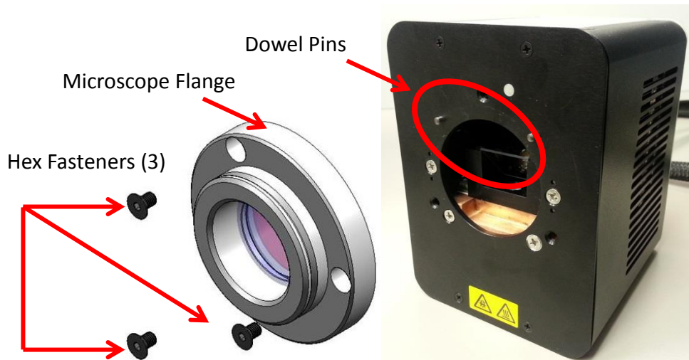
Figure 4 Installing Microscope Flange on LED Head
