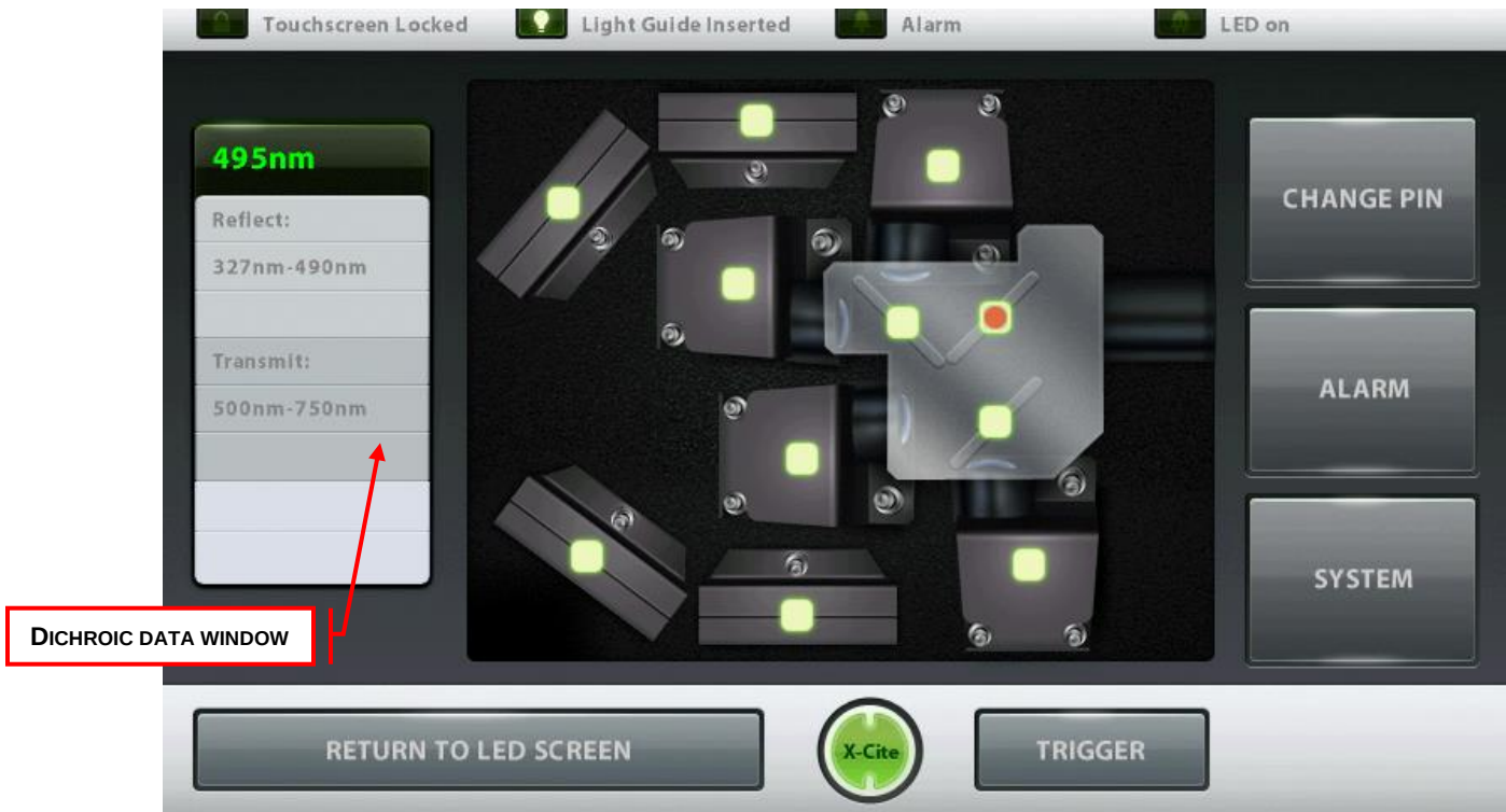
Figure 26 Maintenance Screen (Dichroic Data) (Touch Screen Controller)
