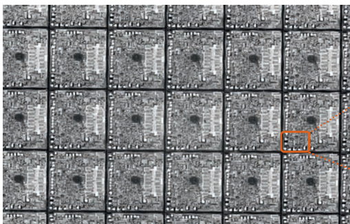
Circuits on silicon wafer grabbed with d.fine HR 3.33x lens + area scan module, camera: 86 MP
