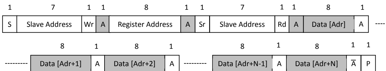
Figure 13: Register read format
