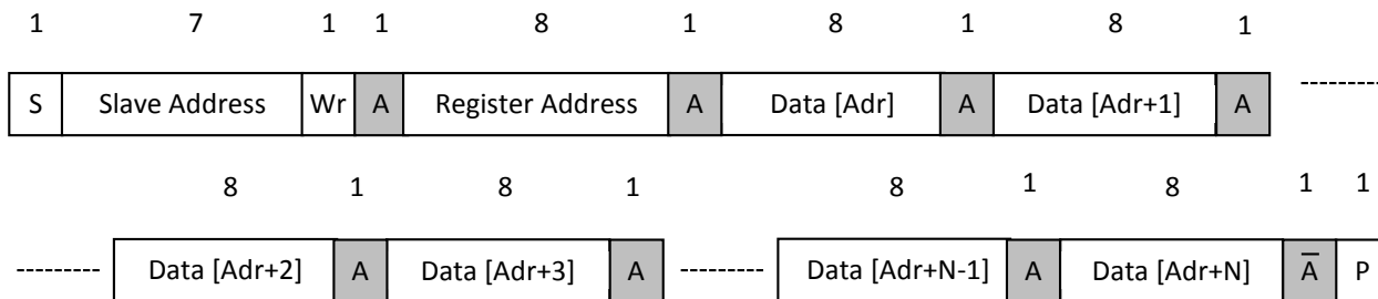
Figure 14: Register write format
