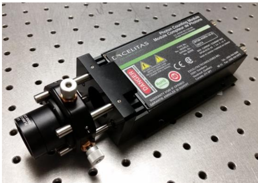
SPCM-AQRH-WX-BR1: with bracket for 1" tube (1.035" x 40TPI) and 30mm cage mount
