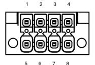
1: Power: V\_in (16-36 VDC / 2A) 5: Power: GND
