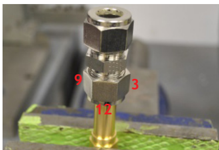
Seat fitting on pipe and mark the 6 O'clock position on nut
