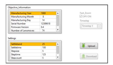
The tabulator called 'Settings' indicates current values and properties. Some refer to the serial interface. Other give the internal temperature inside the Fetura+.
