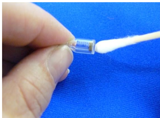
Fig. 5: Cleaning the lamp crystal window
